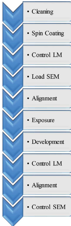
FIGURE 2.13 The process flow of EBL technique.
